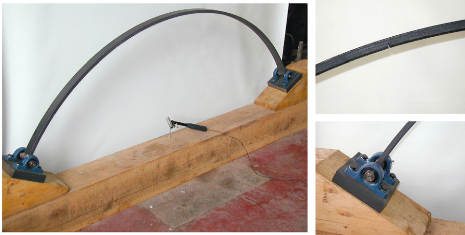
Fig. 1. Circular arch specimen: particulars of the notch and of the hinged end.
